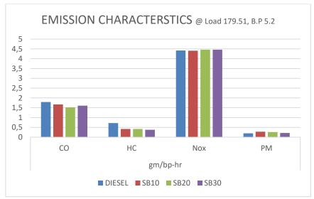
Fig.5 Shows the graph of Emission characteristics at Load 179.51 and B.P 5.2
